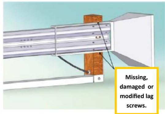
Missing, damaged or modified lag screws.
